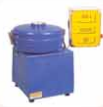
Centrifuge Extractor 1500/3000g capacity
